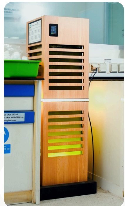
Laboratory Room Plant 1 Jababeka PT Zeus Kimiatama Indonesia (22 x 10 m) Photobioreactor 100L.
